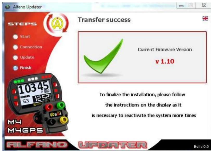
17. Turn on your display (lower right button), and the display will show an operation, validate it by pressing OK (upper right button), the system will resume its update. After operation ends, your display shuts off again, switch it on again (lower right button)
