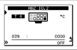
Settle this entry as for the temperature on Box10 (entry « **8/10** »), the only difference, is that you can deactivate this entry « **OFF** ». See page 16.
