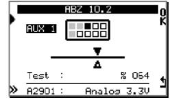
Press on « OK » to show and memorize a mark which will allow to calibrate the graph in the software.
