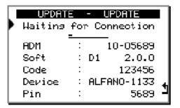
This menu consists in activating Bluetooth to make an UPDATE of the system. All the necessary codes are displayed to synchronize to the computer. ATTENTION: Some computers allow with difficulty a Bluetooth connection, in this case, it's better to use the USB-Bluetooth key supplied with the ALFANO. (See details on chapter Update).
