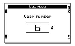
Press on left arrows to select the number of gear that the gear box of the vehicle contains, then, press on « OK » to go on with configuration.
