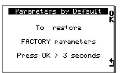
To restore the parameters of factory, press 3 seconds on « OK » to launch the procedure. <u>Note</u>: this procedure does not erase tracks and recorded data.
