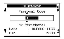
Customize the personal code to protect your data during the connection (code by default « 000000 »). The name of the peripheral and the PIN code cannot be modified, they are unique for every device. <u>ATTENTION</u>: this window does not activate Bluetooth..
