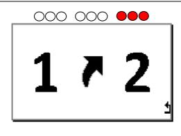
3) The <u>red</u> LEDs replace the <u>white</u> ones. At this moment, the ALFANO asks you to engage the next gear that will be gear 2. Then,
