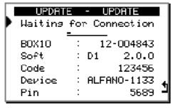
Check the serial numbers of the display and the box. Press on arrow to vary the display of these numbers.
