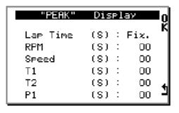
In race, in every detection of level change of the data between the down/up and the up/down of RPM, SPEED, T1, T2, the ALFANO allows to freeze these values in the screen during a scheduled lapse of time, this to have time to visualize them.
