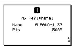
A window appears with the necessary information for the synchronization of these two devices. Introduce these data and the configurable personal password in the « SETUP ».
