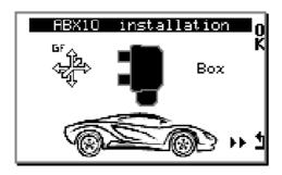
The Box **ABX10** is provided with an integrated 3 dimensional G-Force sensor. It is important to settle the Box correctly on one hand and to configure its position in this menu on the other hand to obtain correct G-Force data. Press on « **OK** » to start the configuration.
