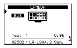
Check the LAMBDA sensors (option) connected on BUS entries. Press on left arrow to commute to the other LAMBDA sensors.
