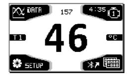
In « WELCOME » page, the temperatures **T1** (bigger, in the display's center) and **T2** (littler, above T1), display after 10 seconds of inactivity of buttons.
