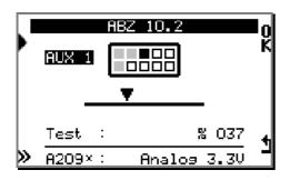
The entries « AUX » allow to measure a movement expressed in percentage by means of an Analog sensor 3.3/5V or of a Potentiometer of 5/10K, for the pedal, the steering wheel, the shock absorber, etc... from 0-100%. Press on arrow >> to choose the type of sensor:
