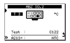
Settle this entry as for the temperature on Box10 (entry « **8/10** »), the only difference, is that you can deactivate this entry « **OFF** ». See page 16.
