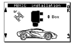
Press on left arrows to display the 4 different positions admitted for a correct installation of the box on the vehicle. Then, press on « **OK** » to display the next window.
