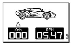
• Engage the first gear and run. (for the karting, this configuration can be made on the trolley). As soon as the ALFANO detects speed and RPM, this window is going to be replaced by the following one. See picture below.
