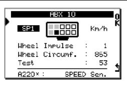
Before setting this menu, it is necessary to connect at first a speed sensor ref. « A220\* » with a magnetized ring to install on the rear axle for karting or little magnets to be fixed on the propeller shaft for cars or a special magnetized support for the motorcycle. Then, press on « OK » to start the setting.
