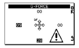
This window shows the G-Force values on 4 directions on real time. The check is made vehicle in the stop and it is important to place the vehicle very horizontally on one hand and to adjust finely the position of the box on the other hand (by respecting the orientation chosen in the previous menu), to obtain the G-Force values bordering the Zero.
