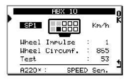
This menu is a direct access allowing to set the parameters of speed in the Box **ABX10 « SP1 »** and in the Box **ABZ.2 « SP2 ».** Press on arrow to chose between:
