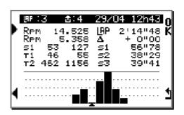
The cursor positions automatically on the best lap, barsgraphs represent the number of laps and the height indicates the difference of time between every lap. The gap of time between the low level and the top level of bars-graphs is customizable in the menu « SETUP »
