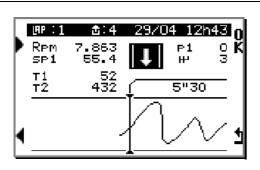
For an accurate analysis, this option allows to view the chosen lap on (step 2), step by step, according to the recording frequency chosen on« SETUP » : RPM (+graphic), SPEED, T°1, T°2, PRESSURE P1, GEAR ENGAGED, DIRECTION OF VEHICLE. Use the arrows to browse the lap, a long pressure allows a fast scrolling.
