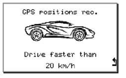
You have to run to more than **20 kph** because the ALFANO also has to memorize the sense of running of the vehicle while recording the GPS coordinates.
