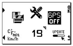
To reactivate the GPS module, press on « **OK** » on icon "**GPS OFF**", then press again 3 seconds on « **OK** » in the window of confirmation which follows. ATTENTION: The ALFANO switches off automatically, then switch it on to validate the change. <u>Note</u>: the consumption of the GPS module decreases the autonomy of the batteries of +/-40 %.
