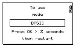
3 seconds pressure on « **OK** » in this window of confirmation to reach the **BASIC** way of working. See chapter, « BASIC mode, page 37 ». ATTENTION: the ALFANO switches off automatically after doing a data erasing, then switch it on again to validate the change.
