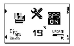
If in some cases, the GPS is not necessary, you can deactivate it. Presss on « **OK** » on icon "**GPS ON**", then press again 3 seconds on « **OK** » in the window of confirmation which follows.
