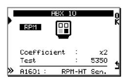
This menu is a direct access allowing to settle the parameters of the RPM.
