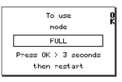
Then press 3 seconds on « **OK** » in the window allowing to go back on FULL mode. ATTENTION: the ALFANO switches off automatically after doing a data erasing, then switch it on again to validate the change.
