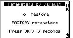
Restore the parameters of factory, press 3 seconds on « OK » to launch the procedure. <u>Note</u>: this procedure does not erase tracks and recorded data.
