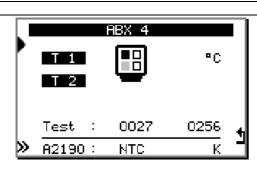
Possibility of connecting 2 sensors with the Y cable « A2190 ». Press on arrow >> to make your choice :
