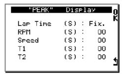
In race, in every detection of level change of the data between the down/up and the up/down of RPM, SPEED, T1, T2, the ALFANO allows to freeze these values in the screen during a scheduled lapse of time, this to have time to visualize them.
