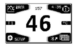
In « WELCOME » page, the temperatures **T1** (bigger, in the display's center) and **T2** (littler, above T1), display after 10 seconds of inactivity of buttons.
