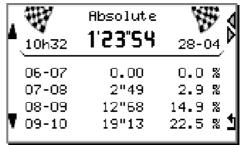
Press the arrow to show next window, RPM ranges. This option allows to analyze the behavior of the engine through RPM ranges, that is to say the time + the conversion in percentage of this time for all the RPM ranges of 1.000 rotations/min accumulated in this lap. Press on « » to show the next RPM ranges. Press on double arrow to vary and so compare the data of these two laps. Press on « » to go back on menu DATA.
