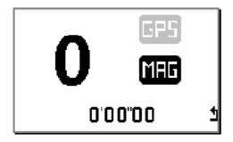
This window appears as soon as the vehicle exceeds **20 kph**. The icon « **GPS** » is not active, because the ALFANO has to get first and foremost the magnetic strip.
