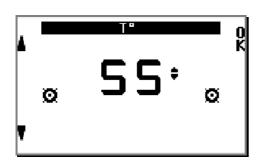
• Settle the threshold of the 2 leds for the Temperature **T1**
