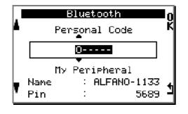
Personalize the personal code to protect your data during the connection (code by default « 000000 »). The name of the peripheral and the PIN code cannot be modified, they are unique for every device. <u>ATTENTION</u>: This window does not activate Bluetooth.
