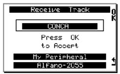
The name of the track to receive appears, press on « **OK** » to accept the track.
