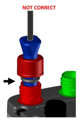
the female connector before tightening the nut.
