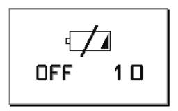
When this message displays, M4/M4GPS goes automatically off after 10 seconds.
